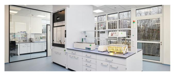
An innovative air concept integrates the Köttermann fume cupboards into the ventilation and temperature control system, thus contributing to consistent laboratory air quality. The fume cupboards therefore fulfil a dual function: they not only protect employees during critical work steps, but also ensure a healthy room climate through air exchange.
